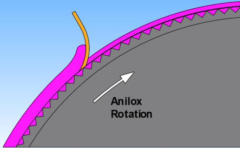
Thicker doctor blades will resist deflection from extra pressure forces and provide a controlled, clean wipe of the surface of the anilox.
