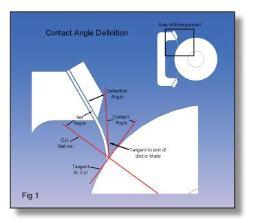
angle, other than running the chamber at the minimum applied pressure required to maintain a clean, uniform wipe.
