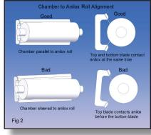
gage between the doctor blade and anilox roll on one end. Set the chamber position so that the feeler gage will slip between the blade and anilox roll with slight tension. Now check the gap between the rest of the blade and anilox roll. It should be the same everywhere on the blade and the same on the containment blade. Adjust the chambers position as necessary until there is uniform gap on both blades.
