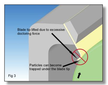
excessive pressure will increase the wear on the blade and anilox roll—both of which are undesirable.
