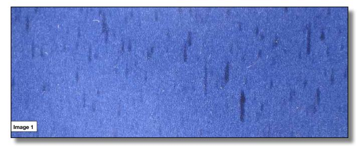
the footprint—the area of steel in contact with the anilox roll—will increase, thereby increasing the potential for ink to get past the doctor blade. Although not indicated in the chart, the material tested was a long life tool steel with a laser hardened working edge. The extra hardness provided by the laser further reduces blade wear and helps to prevent the working edge of the blade from over deflecting.
